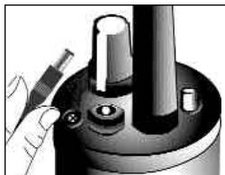
Transmitter charger and charging jack
