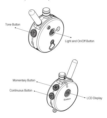
The ET-800 transmitter is equipped with four control buttons, LCD display, and an adjustable dial. For long range use hold the transmitter up like the Statue of Liberty and never allow the antenna to touch anything as it will decrease the range. Power lines and foliage will also reduce the range.
