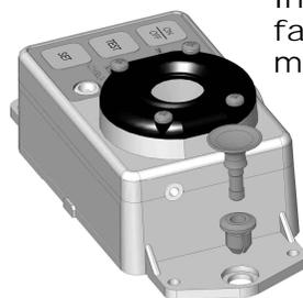
Installing Nylatch fasteners on receiver mounting plate.
