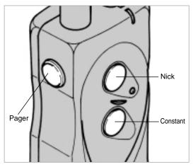
The transmitter for **dogtrd 2200NCP** has three buttons (two on the face of the transmitter and one on the side).
