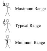
If your finger touches the antenna near the dial on the top of the transmitter, the actual range may be reduced. Additional environmental factors may also affect the range of your unit.
