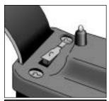
Protection cap not fitted properly. Moisture and debris can enter charging jack.
