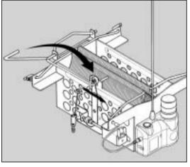
Figure 5. Setting the latch.
