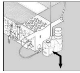
Figure 1. Mounting the receiver
