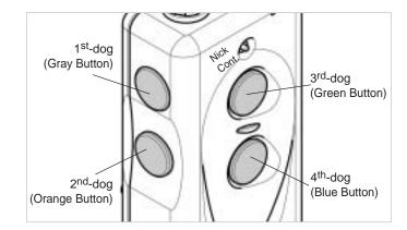
**The transmitter for the** *dogtrd 1804NC* **has four buttons;** The Gray (1<sup>st</sup> dog) button corresponds to the receiver with the black collar strap. The Orange (2<sup>nd</sup> dog) button corresponds to the receiver with the orange collar strap. The Green (3<sup>rd</sup> dog) button corresponds to the receiver with the green collar strap. The Blue (4<sup>th</sup> dog) button corresponds to the receiver with the blue collar strap.
