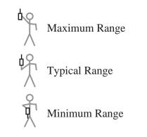
If your finger touches the antenna near the dial on the top of the transmitter, the actual range may be reduced. Additional environmental factors may also affect the range of your unit.
