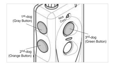
**The transmitter for the** *dogtra***1803NC has three buttons;** The Gray (1<sup>st</sup> dog) button corresponds to the receiver with the black collar strap. The Orange (2<sup>nd</sup> dog) button corresponds to the receiver with the orange collar strap. The Green (3<sup>rd</sup> dog) button corresponds to the receiver with the green collar strap.
