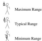
If your finger touches the antenna near the dial on the top of the transmitter, the actual range may be reduced.
