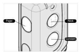
The transmitter for **dogtrd 200NCP GOLD** has three buttons (two on the face of the transmitter and one on the side).
