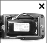
\* Caution - The battery wires must be inside the battery compartment tucked neatly along the right side of the battery.
