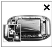
\* Caution - The battery wires must run neatly along the top left side in to the battery compartment.
