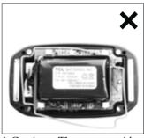
\* Caution - The orange rubber gasket is important for the unit to be waterproof and must be properly seated in place.
