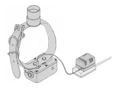
To charge the battery, plug the charger into the battery receptacle on the collar and plug the adapter into any standard 110 Volt household wall outlet. (A 220 Volt European adapter is available from D.T. Systems). Recharge the battery for no more than 14 hours. Important: After charging make sure to plug in the rubber receptacle plug firmly to prevent dirt and water from entering the unit.
