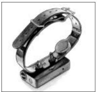
Collar. The waterproof sealed case contains battery-powered electronics. The round, rubber covered disk on the collar strap is a vibration sensor. Electrical stimulation is applied briefly when the
