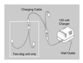
The battery charger and charging cables allow you to charge both the transmitter and receiver at the same time. The battery charger is designed for a 120 volt wall outlet. (European 230 volt AC chargers and 12-volt field charger for your automobile are also available.)
