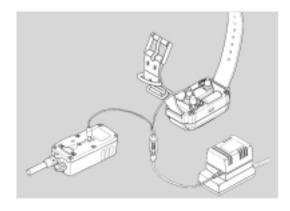
dogtra uses Ni-MH (Nickel-Metal-Hydride) batteries that do not set a memory and can be charged on a regular basis without harm to the battery. There is no need to completely drain the batteries between charges. However, doing so will help to extend the overall lifetime of the batteries.
