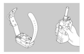
1. Turn the collar on by pressing the button on the back side of the collar receiver. The indicator light will come on for a moment then blink once every two seconds, showing that the collar is ready to use. (If the indicator light is red, the batteries need to be charged.) Place the test light on the contact points of the receiver and hold it there.
