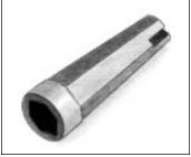
before each use. The contact points must be more than finger-tight. Be certain to use only the contact point wrench to tighten the contact points.
