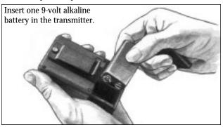
**Important:** The positive and negative terminals of the transmitter batteries must match the positive and negative contacts in the battery compartment.
