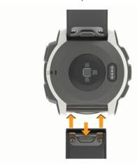
**NOTE:** Make sure the band is secure. The latch should close over the watch pin.
