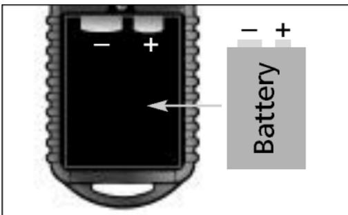
The larger battery terminal should touch the larger transmitter contact.
