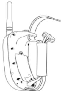
3. Thread loose end (non-buckle end) of the strap through the top guide.
