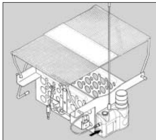
Figure 2. Plugging solenoid cord into the receiver.
