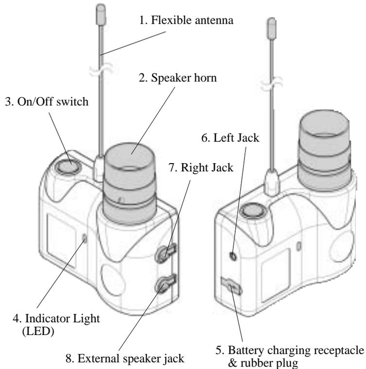
**1. Flexible antenna** : Flexible antenna is located on the top of the receiver. Please do not bend the antenna forcibly for it can cause serious reduction in range.
