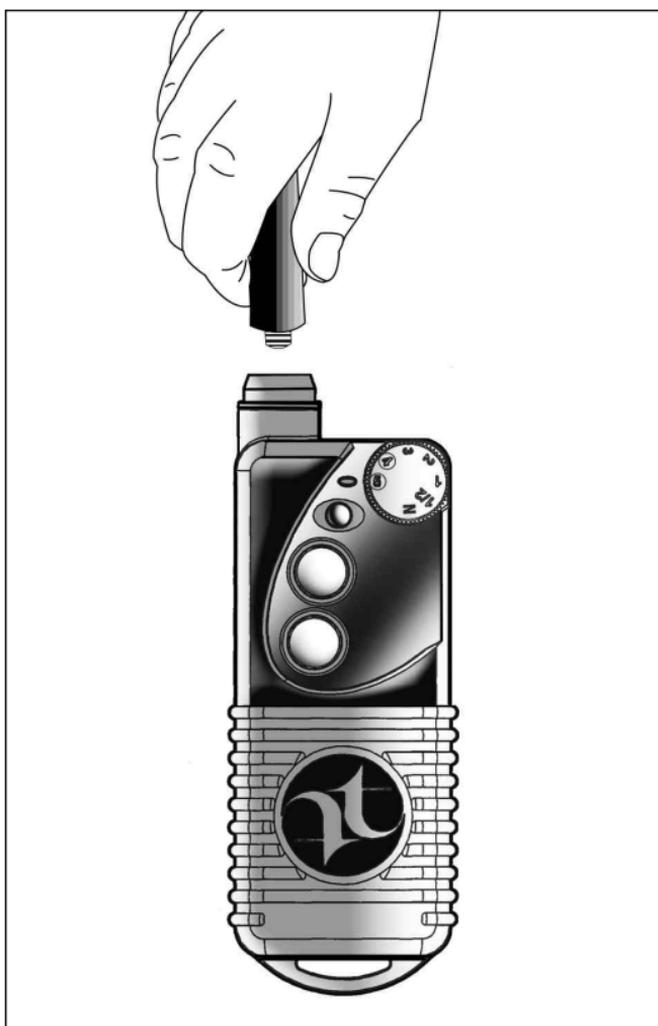
Hold the antenna near its base and tighten by hand.
