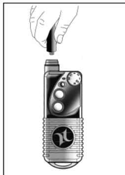
Hold the antenna near its base and tighten by hand.
